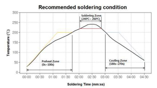
Recommended Re-flow Temp & Speed Max 260 Degree 0.6m/Minute
